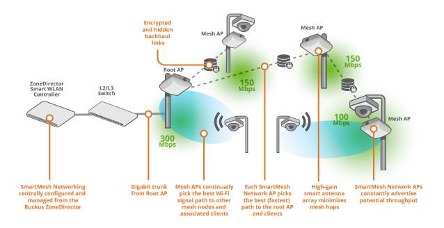
Figure 1. SmartMesh Networking with wireless video surveillance cameras
